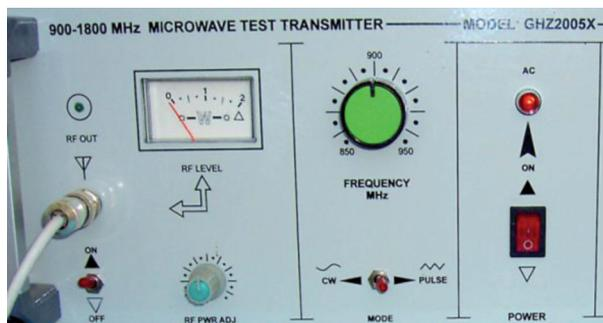
**Figure 1.** Electromagnetic energy generator which produced 900 MHz EMF like mobile phone frequency (Set Elec.Co. Istanbul / Turkey)
