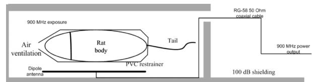
**Figure 3.** 900 MHz EMF Exposure system
