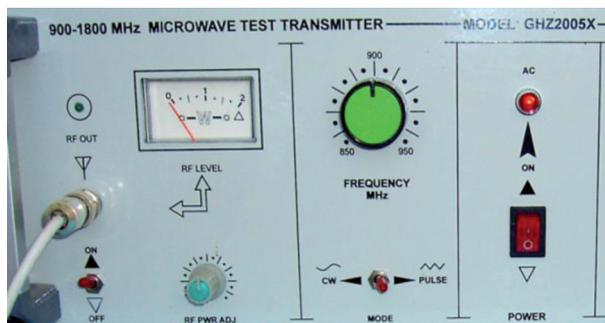
**Figure 1.** Electromagnetic energy generator which produced 900 MHz EMF like mobile phone frequency (Set Elec.Co. Istanbul / Turkey)
